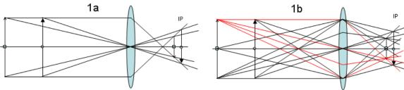
Figure 1. Ray Tracing a Thin Lens
